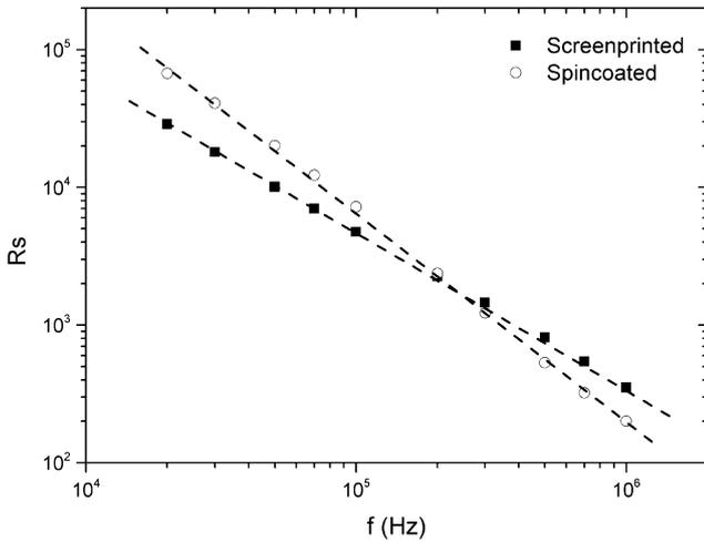
Figure 5. The series resistance,  $R_s$  vs frequency,  $f$  plot of Al/PAN/p-Si screen printed and spin coated devices.
