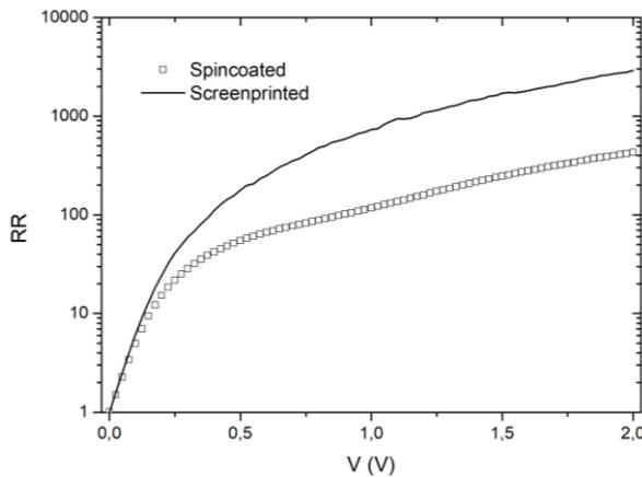
Figure 2. The graph of Rectification Ratio vs. Voltage of Al/PAN/p-Si spin coated and screen-printed devices in a semi-log I-V plot.
