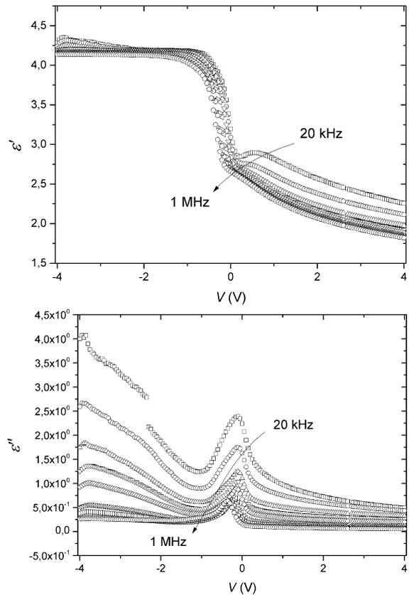
Figure 6. The dielectric measurements of Al/PAN/p-Si spin coated device.
