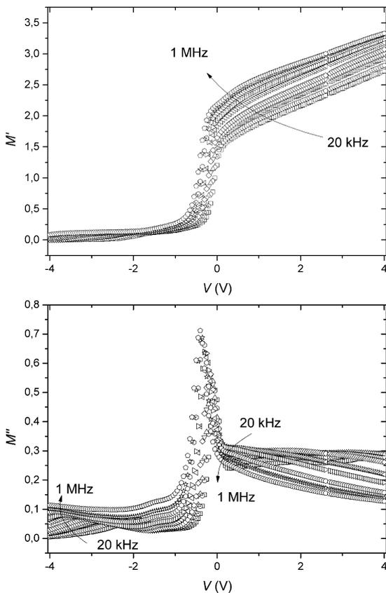
Figure 10.  $M'$  and  $M''$  -  $V$  graphs of Al/PAN/p-Si screen-printed device.
