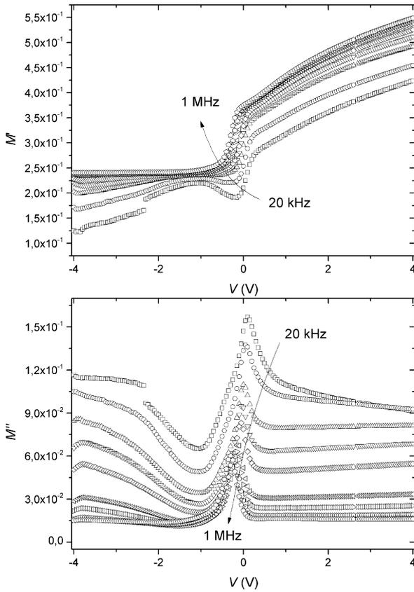
Figure 9.  $M'$  and  $M''$  -  $V$  graphs of Al/PAN/p-Si spin coated device.
