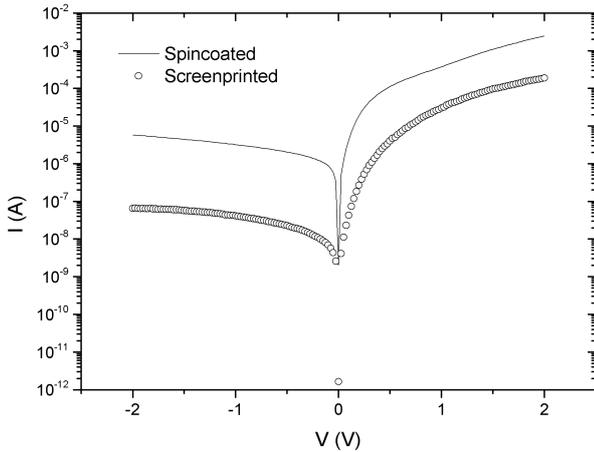
Figure 1. The Current vs. Voltage graph of measurements of Al/PAN/p-Si spin coated and screen-printed devices in semi-log I-V plot.
