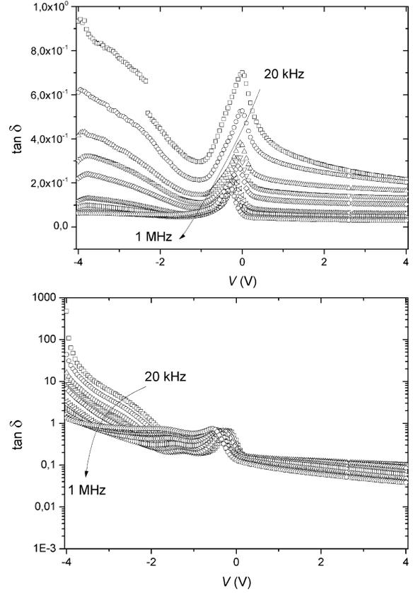
Figure 8.  $\tan\delta - V$  graphs of Al/PAN/p-Si spin coated (top) and screen-printed (bottom) devices.
