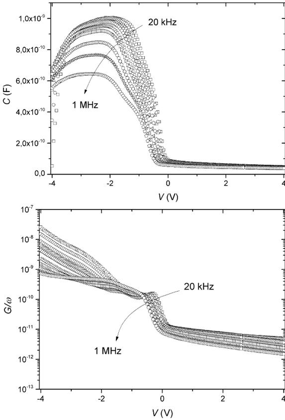
Figure 4. C-V and G/ω-V plot of Al/PAN/p-Si screen-printed device.
