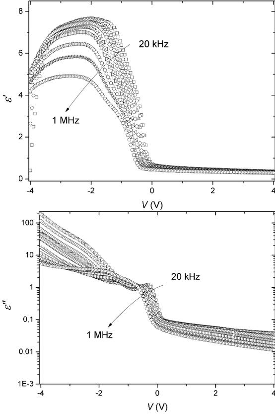
Figure 7. The dielectric measurements of Al/PAN/p-Si screen-printed device.
