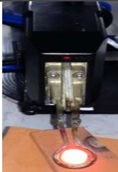
Figure 2. Induction sintering process of the iron based PM compact
