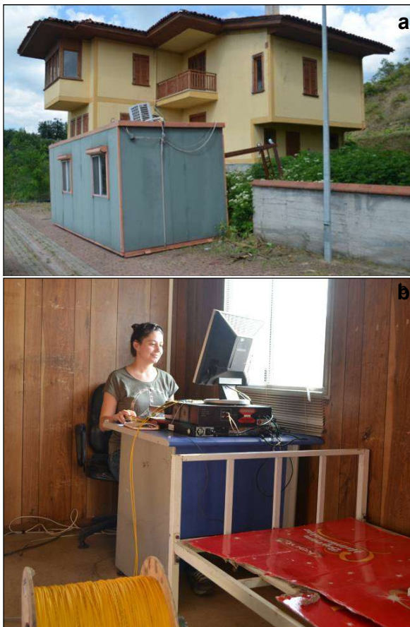
Fig. 6. a) The container's location behind the crown of the landslide b) An inside view of the container and the optical fiber system components.
