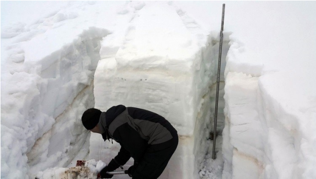
Figure 9. Snow Pit on Bozdağ North Face and Simple Snow Stability Tests (Dr. E. Tekin-2015)
