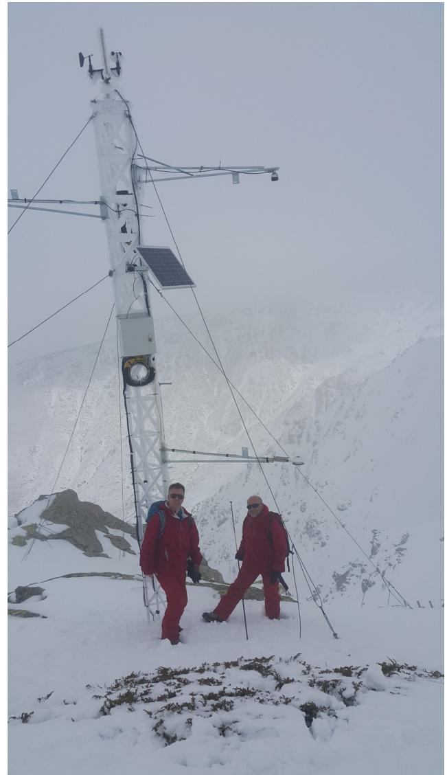
Figure 10. Automated Weather Station For Avalanche Studies on Bozdağ Summit (Ö. Koçyiğit and G. Arslan-2016)
