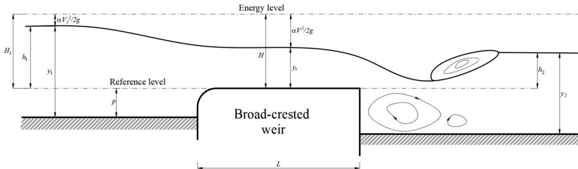
Figure 1. Flow over a broad-crested weir (Bos MG, 1976)
