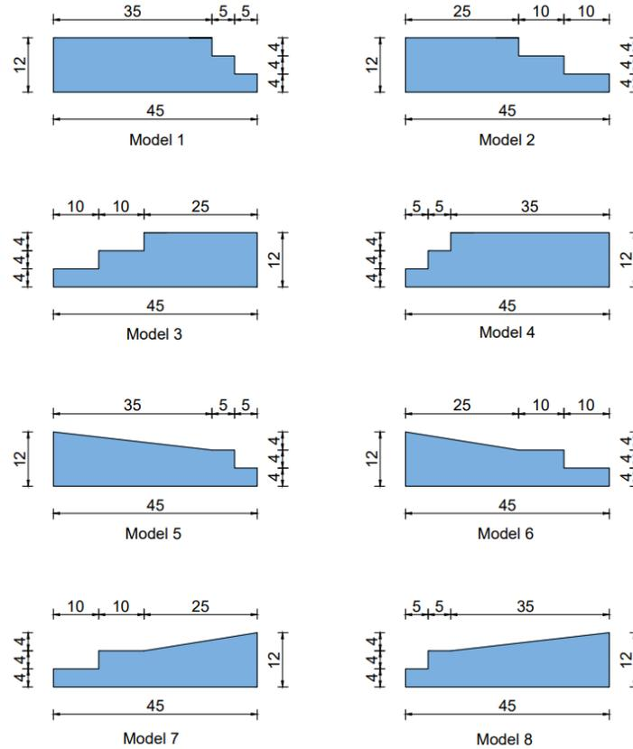
**Figure 3.** Designed models (all measurements are in cm)
