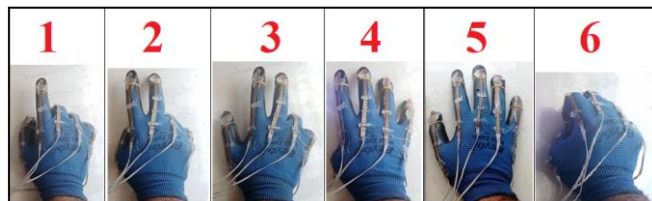
Fig.2. Hand gesture recognition from sensor arrays based on flex sensor
