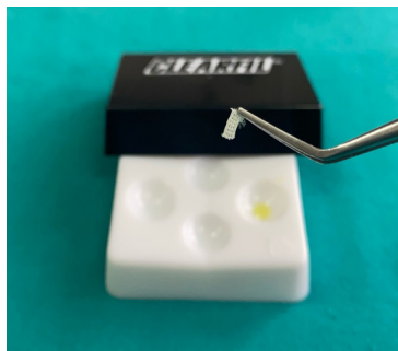
Figure 3. Fiber material and bond agent cut according to mold dimensions before saturation process
