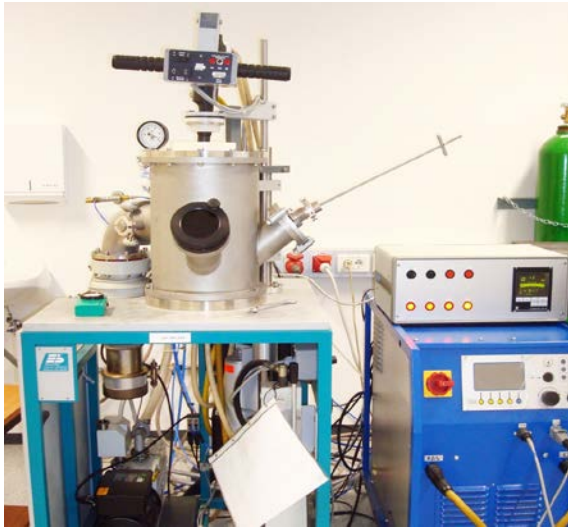
Figure 1. Edmund Buehler Arc Melter furnace
