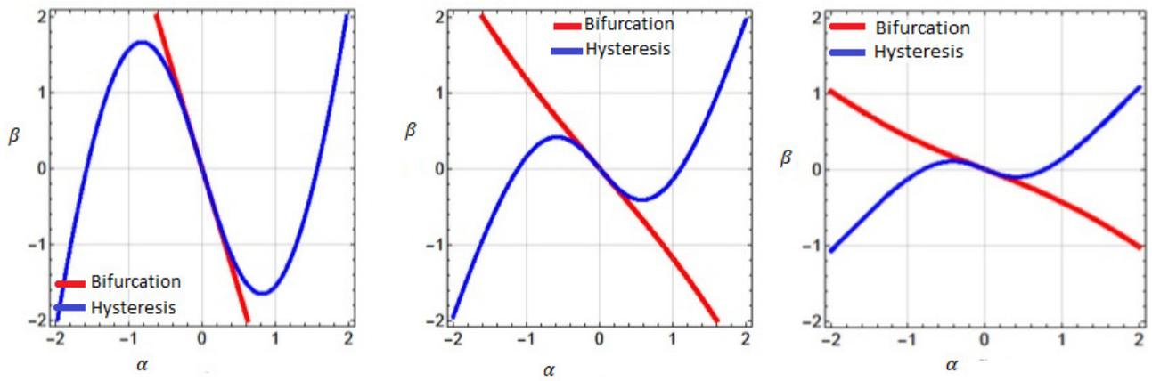
Figure 3.  $B$  and  $H$  ( $a_0 = 2, a_{\alpha, \beta \geq 1} = 0$ ) estimates in  $\alpha\beta$  plane
