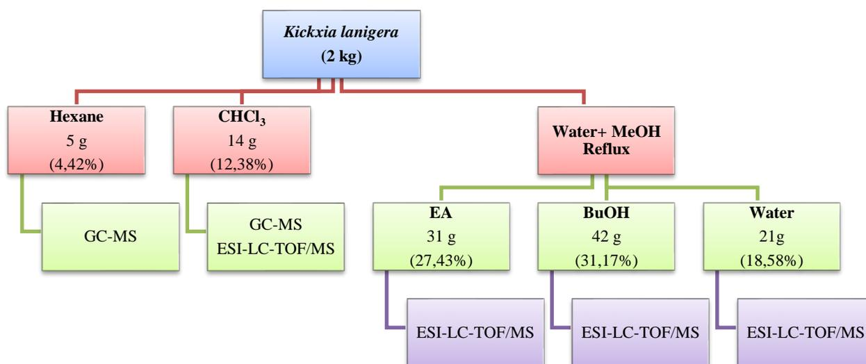
**Figure 2.** Extraction and analysis scheme of *K. lanigera*
