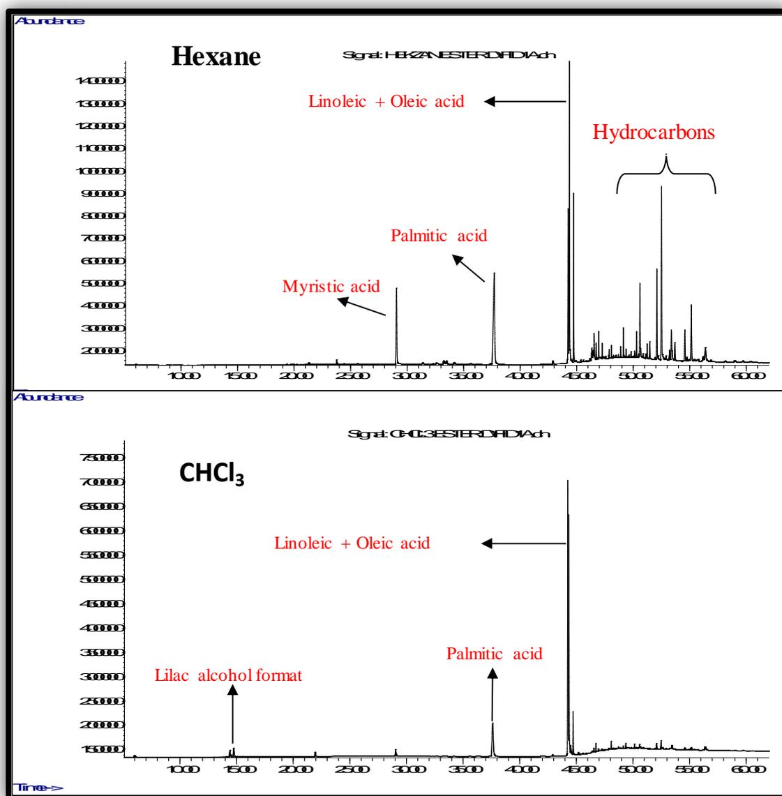
**Figure 3.** FID chromatograms of hexane and CHCl<sub>3</sub> extracts of *K. lanigera*
