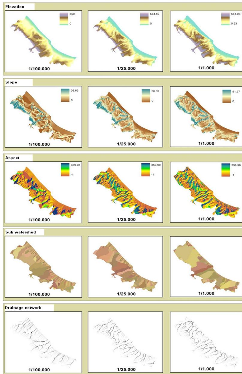
**Figure 11.** The comparison of DEM, Slope, Aspect, Watershed and Drainage networks obtained in 50 m pixel size from 1/100.000, 1/25.000 and 1/1000 scale map data.
