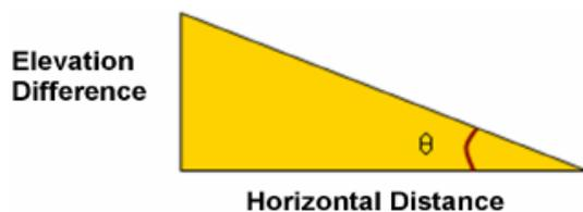
$$\tan \theta = \frac{\text{Elevation Difference}}{\text{Horizontal Distance}}$$
