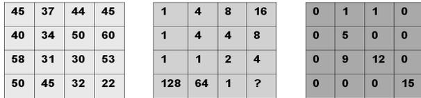
Figure 3. DEM, Flow Direction, Flow Accumulation [25]
