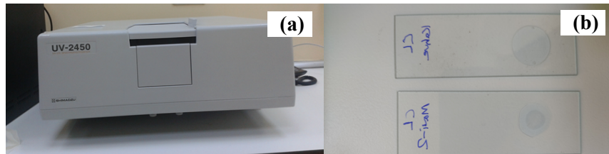
Figure 1: (a) UV-visible spectrometer used for optical absorption measurements of contact the lenses, (b) Examined lens samples
