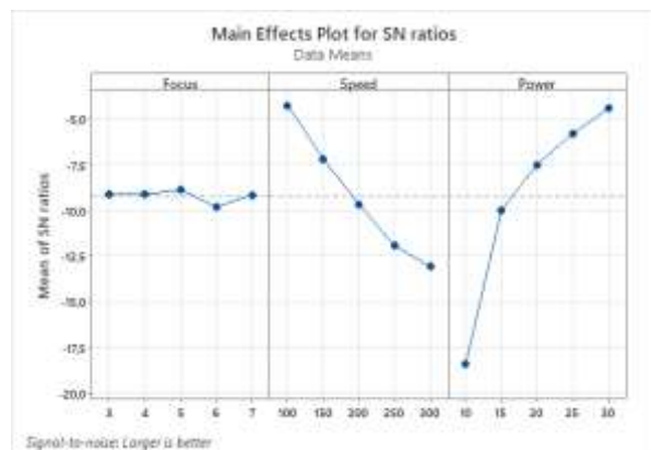
Figure 6. Effect of laser cutting parameters on the scraping depth (SN ratios).
