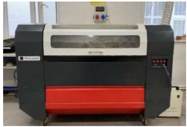
Figure 1. CO 2 laser machine used in the engraving process.
