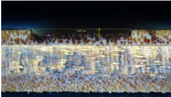
Figure 4. Wood plywood milling depth (D) and determined milling width.
