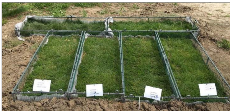
Figure 3. Basket with a size of 1.3m x 0.5m x 0.2m in which rootzones were placed
