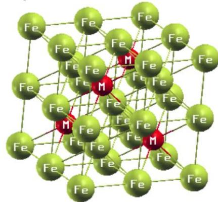
**Fig. 1.** The three dimensional (3D) crystallographic representation Fe<sub>3</sub>M (M=Al, Ga, Si and Ge) full-Heusler alloys in DO<sub>3</sub>-type structure with *Fm* $\bar{3}$ *m* space group.
