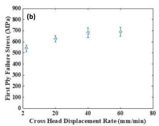
Figure 6: First ply failure, a) Strain, b) Stress
