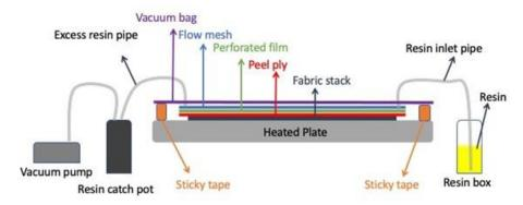
Figure 1: Schematic of the vacuum-influsion process and order of consumables used in the production of the composite test plate
