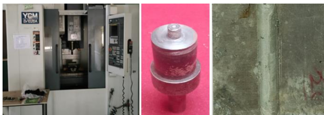
Figure 2. CNC machine, tool, and FSPed specimen
