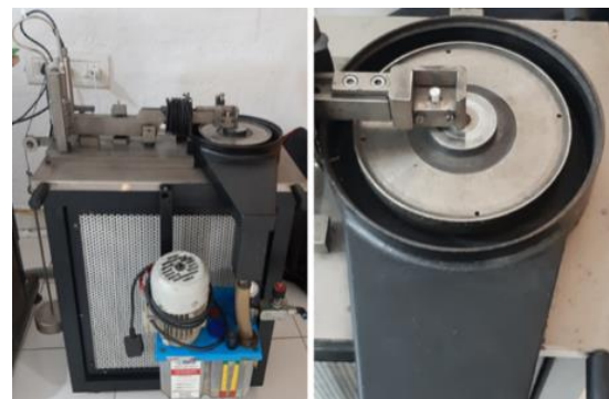
Figure 3. PoD apparatus and pin setup
