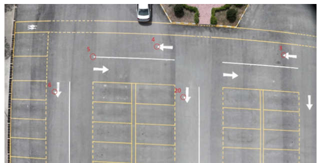
Figure 2 West side of the parking lot from 30 m flight altitude. CPs on this part of the field were marked with red circles (CPs 3-6 and 20).
