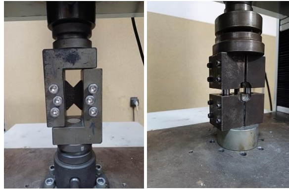
Figure 9. Shear and Compression Test Apparatus
