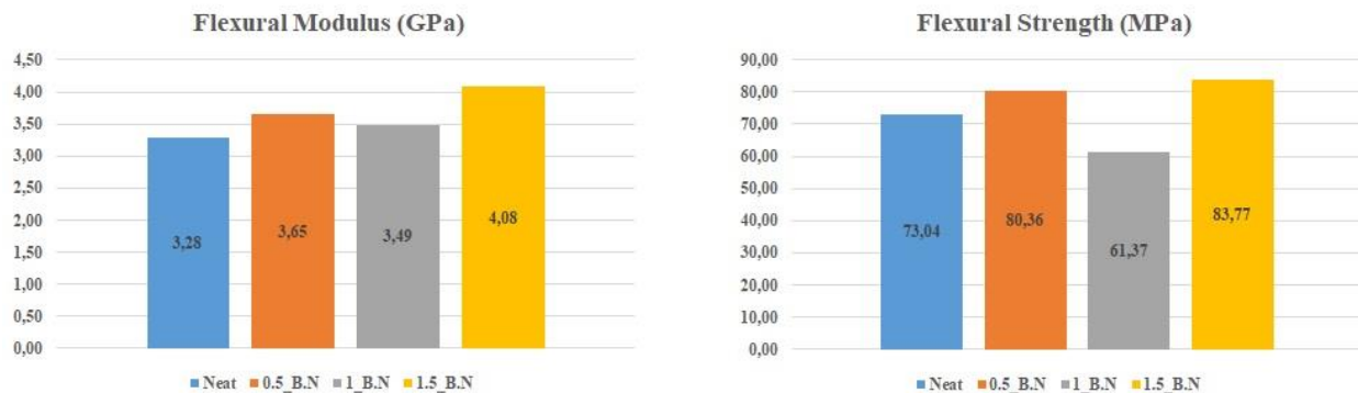
Figure 11. Comparison of Bending Modulus and Bending Strength with Variation in Weight Percentages of (h-BN)
