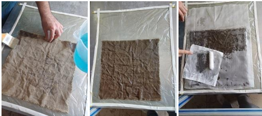
Figure 5. Application of (h-BN) Nanopowder Reinforced Epoxy Resin onto Flax Fabrics by Hand Lay-Up
