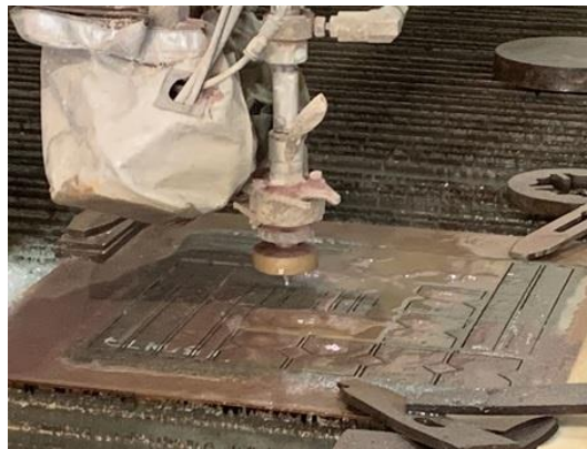
Figure 7. Cutting of Composite Plates to Testing Standards Using Water Jet
