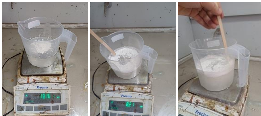
Figure 3. Addition of Hexagonal Boron Nitride (h-BN) Nanopowders in Different Weight Ratios into Epoxy Resin
