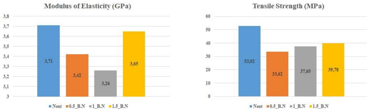
Figure 10. Comparing to Modulus of Elasticity and Tensile Strengths of Epoxy Composites with Varying Weight Percentages of (h-BN)
