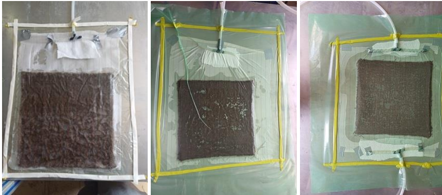
Figure 6. Production of Composite Plates Using the Vacuum Bagging Method
