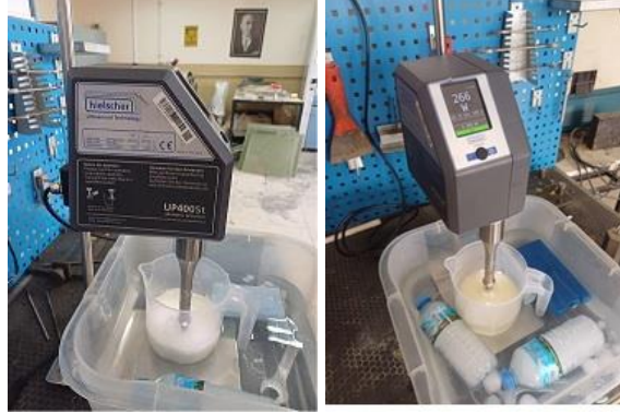
Figure 4. Mixing of Hexagonal Boron Nitride into Epoxy Using an Ultrasonic Mixer
