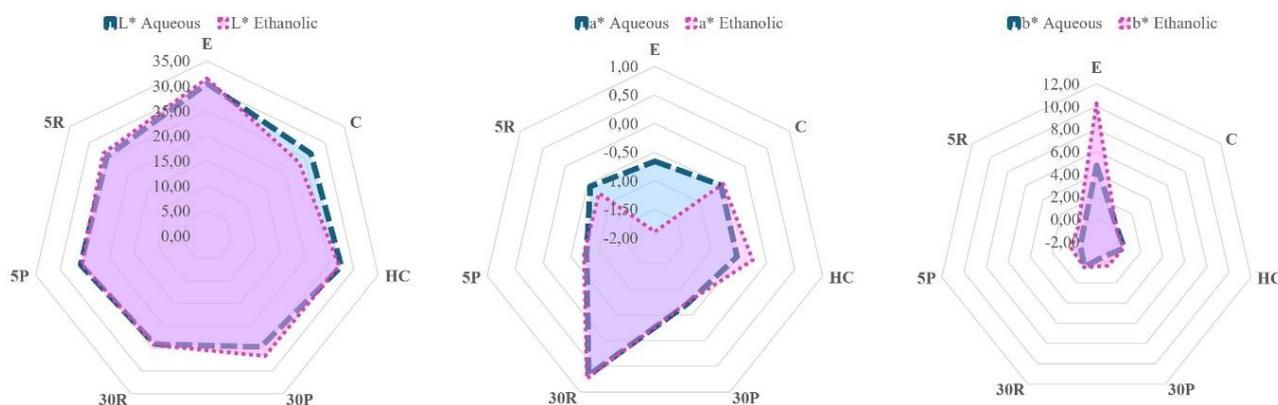
**Figure 2.** Color changes in aqueous and ethanolic stevia extracts throughout processing stages (E: Extraction, C: Centrifugation, HC: Hot clarification, 30P: Ultrafiltration, 30 kDa-permeate flux, 30R: Ultrafiltration, 30 kDa-retentate flux, 5P: Nanofiltration, 5 kDa-permeate flux, 5R: Nanofiltration, 5 kDa-retentate flux).
