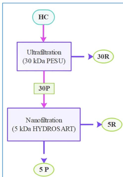
**Figure 1.** Stepwise membrane filtration procedures.
