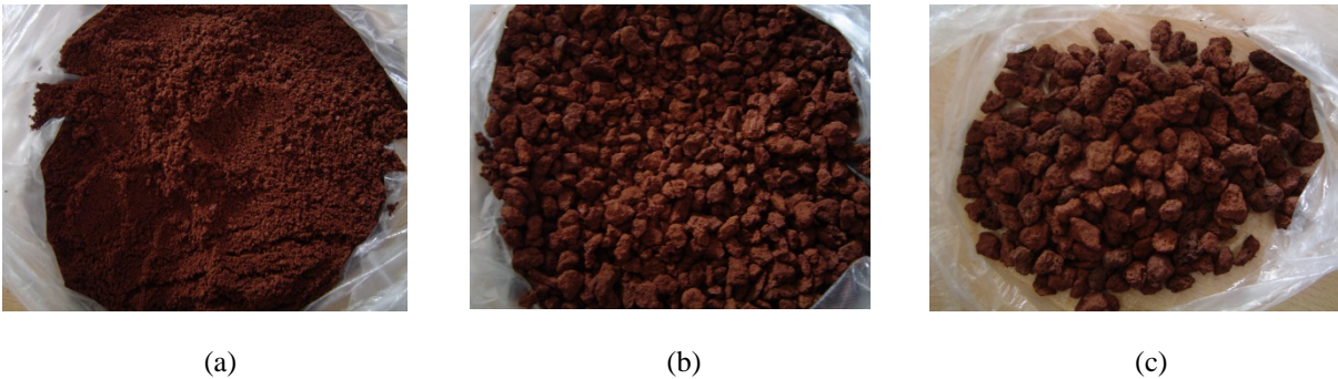
Şekil 1. Denemede kullanılan farklı boyutlardaki pomza örnekleri (a) İnce pomza (0-4 mm), (b) Karışık pomza (4-8 mm), (c) İri pomza (8-16 mm). Figure 1. Examples of different sizes of pumice used in the experiment (a) small pumice (0-4mm), (b) Mixed pumice (4-8 mm), (c) large pumice (8-16 mm).
