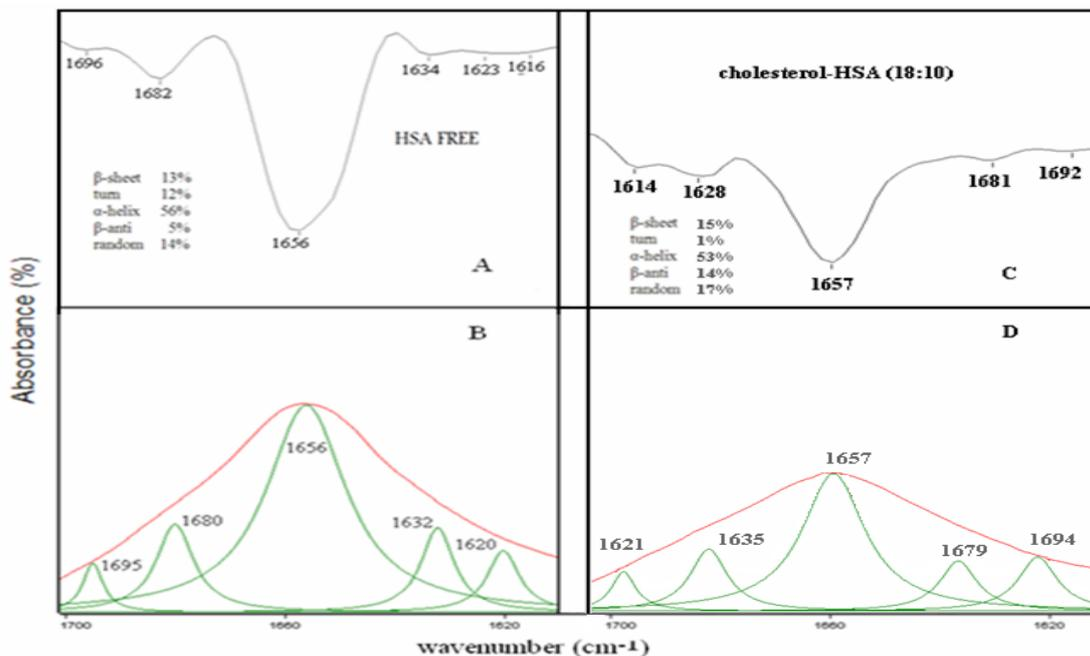
**Figure 10.** Second-derivative enhancement and curve-fitted Amide I region (1610-1700  $\text{cm}^{-1}$ ) and secondary structure determination of the free human serum albumin ( A and B) and it cholesterol complexes ( C and D) with 18:10 cholesterol: HSA ratios.
