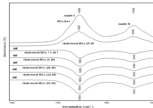
**Figure 8.** FT-IR spectra (top two curves) and difference spectra of HSA and its complexes with different cholesterol concentrations in the region 1800-1500 cm<sup>-1</sup>.
