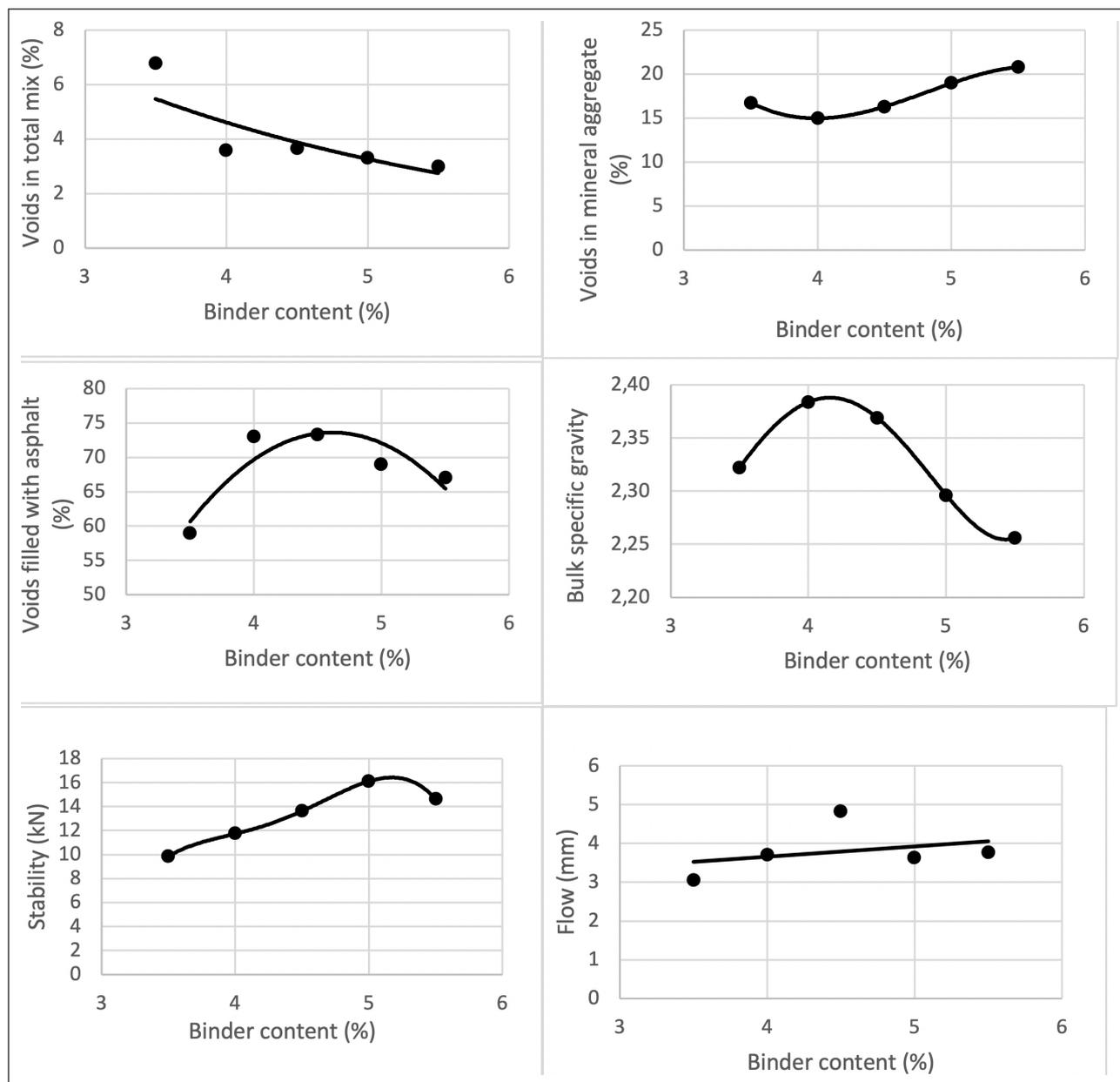
Figure 3. Marshall test results for the control mixture.
