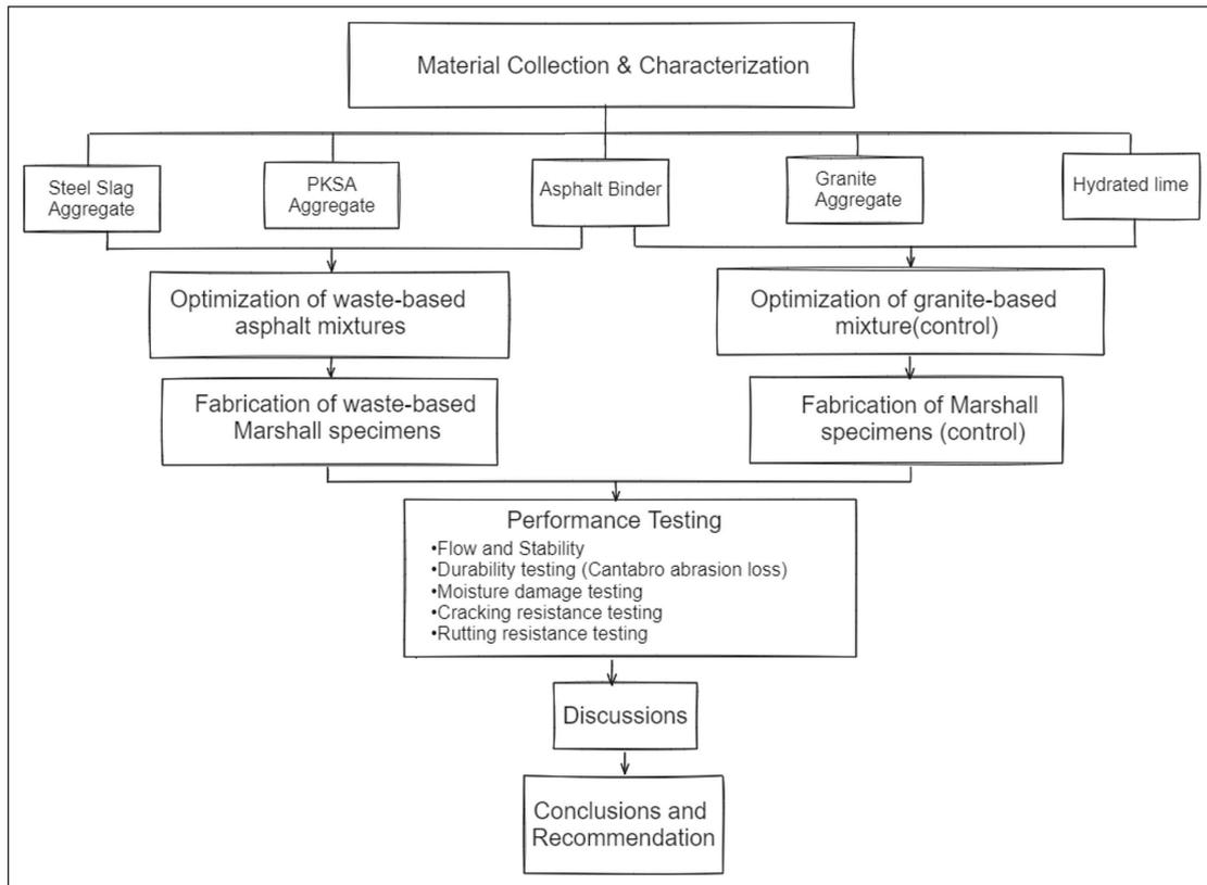
Figure 1. Flow chart of an experimental program.
