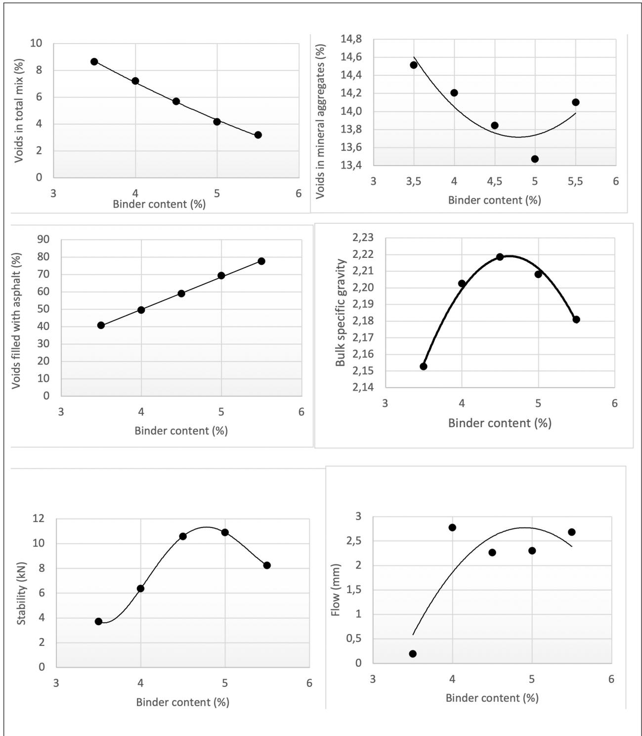
Figure 4. Marshall test results for the waste-based mixture.
