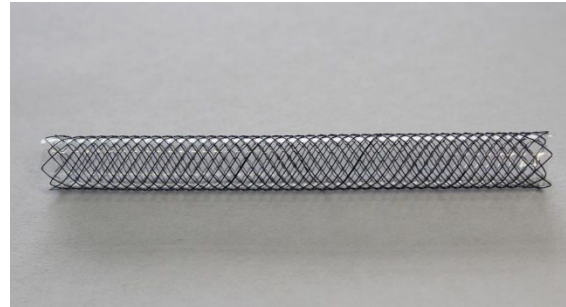
Figure 5. Traditionally manufactured 316l steel stent.
