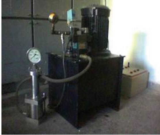
Figure 1. Hydraulic pressure unit.
