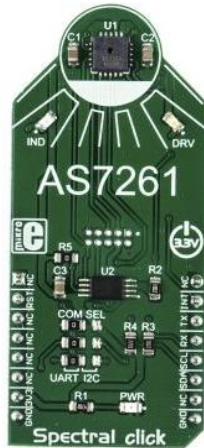
Figure 4. AS7261 XYZ Chromatic White Color Sensor
