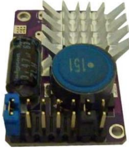
Figure 12. C series constant current LED driver circuit
