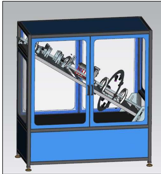
Figure 11. Inspection station and free-fall movement of ammunition cases inside the glass tube
