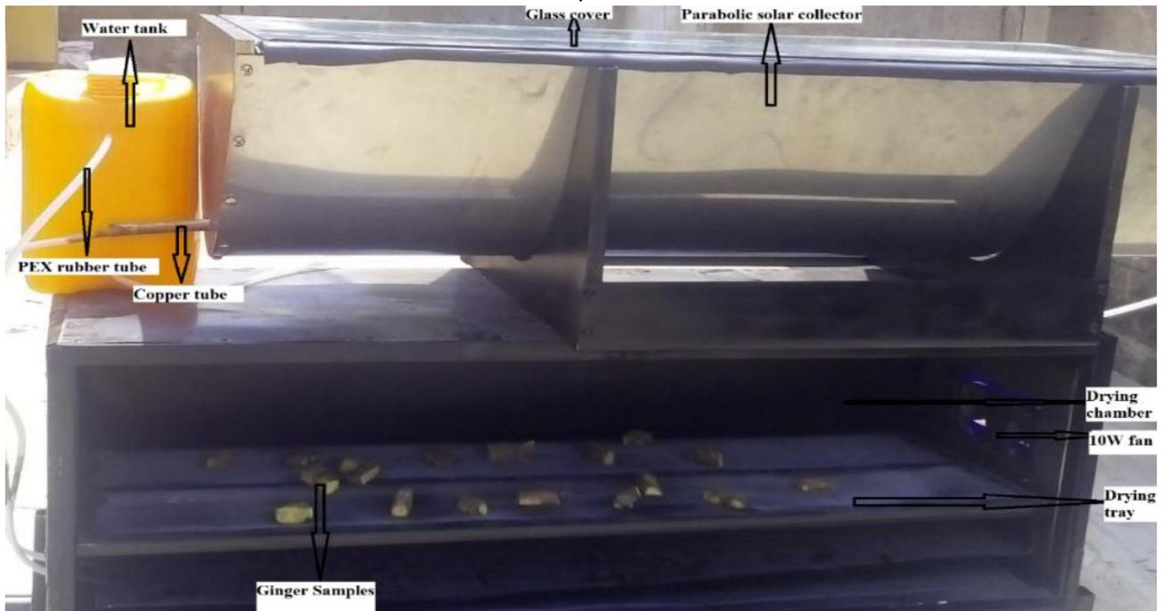
**Figure 2.** Pictorial view of the Experimental setup
