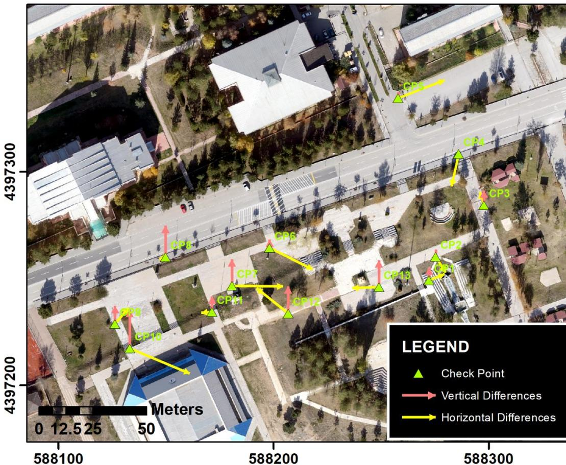
Figure 5. Representation of coordinate differences with vectors (scaled 1/300)
