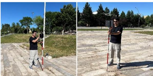
Figure 2. Measurement of check point locations with ViDoc.
