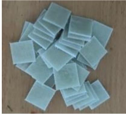
**Figure 1.** Specimen tabs
