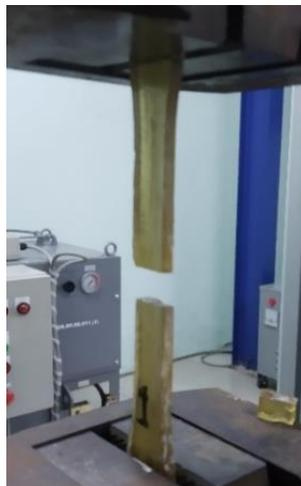
**Figure 7.** Adhesive specimens after the test
