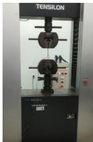
**Figure 3.** Tensile test of adhesive
