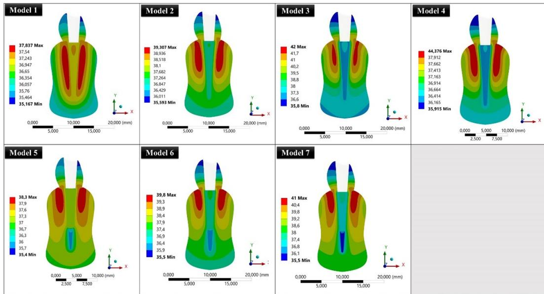
**Figure 5.** The maximum temperatures detected 13 s after the completion of thermoplasticized gutta-percha obturation procedures in the FEA models.
