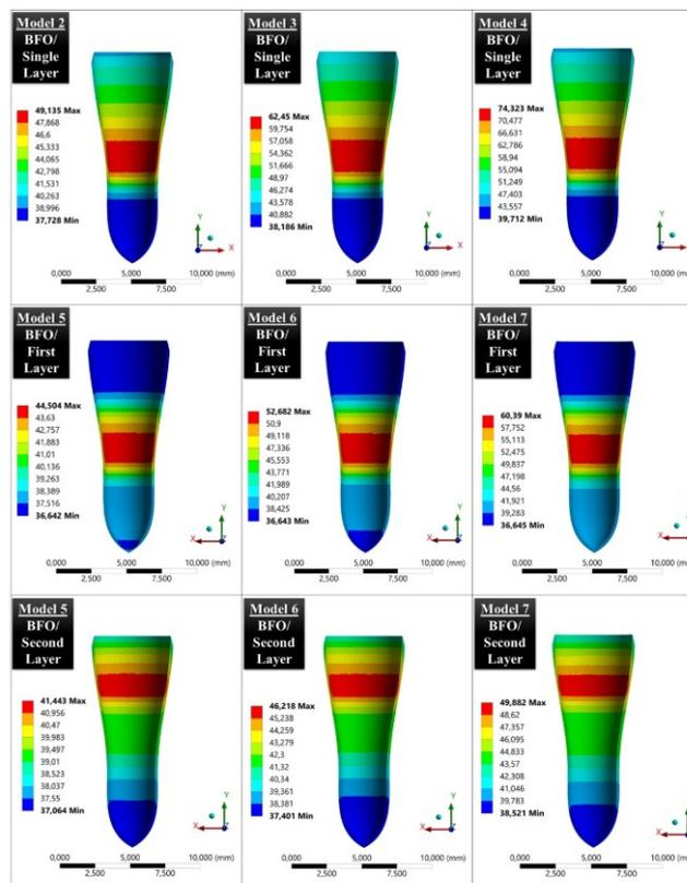
**Figure 4.** Maximum temperatures observed in BFO applications in the FEA models from Model 2 to Model 7.
