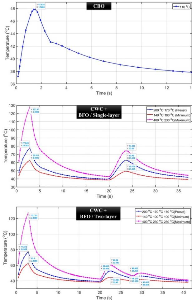
**Figure 2.** Time-dependent temperature changes in periodontal ligament tissue in each FEA model. The initial peaks in temperature represent the application of CWC and CBO techniques, while the second and third peaks indicate the application of the BFO technique for CWC + BFO models, respectively.
