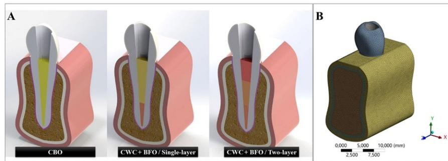
**Figure 1. A)** Finite element models of carrier-based obturation (CBO) and continuous wave of condensation technique followed by backfill obturation (CWC + BFO) techniques. **B)** A meshed model containing elements and nodes.
