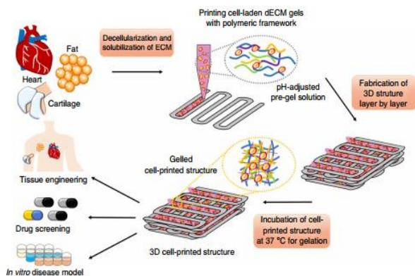
**Figure 8.** Schematic procedure for dECM bioink bioprinting [27].
