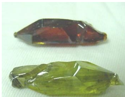
Figure 6. Synthetic ZnO crystals (Red and green colour are associated with different concentrations of oxygen vacancies) [30].
