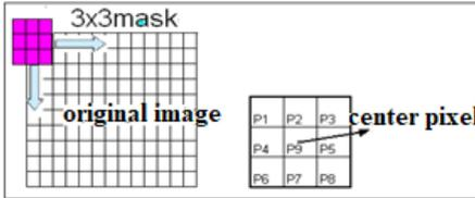
Fig. 1. Place of the mask on the image and location of the center pixel [15]
