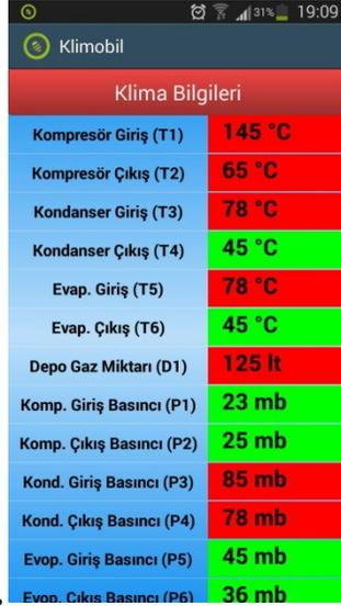
Fig. 10. Screen display showing air conditioner data
