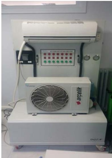
Fig. 4. Air conditioning training simulator system
