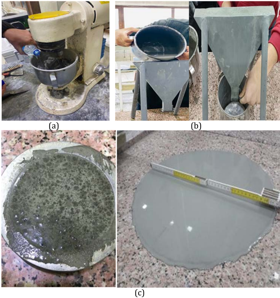
Fig.4. (a) Preparation of mixtures (b) Conducting the mini V-funnel test (c) Conducting the spreading test
