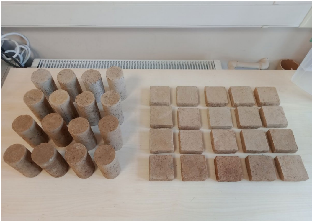
Figure 5. UCS and shear strength test specimens used in this study
