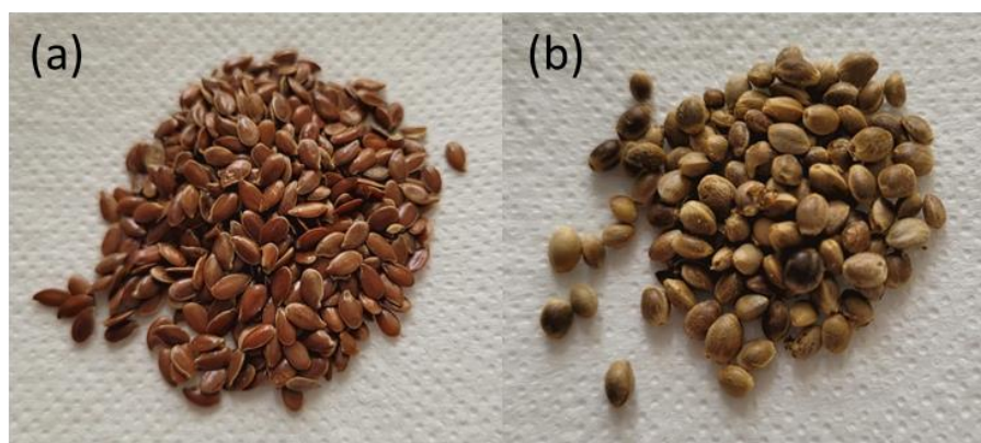
Figure 1. (a) Linseed and (b) hemp seed, whose oils serve as natural self-healing agents in the study
