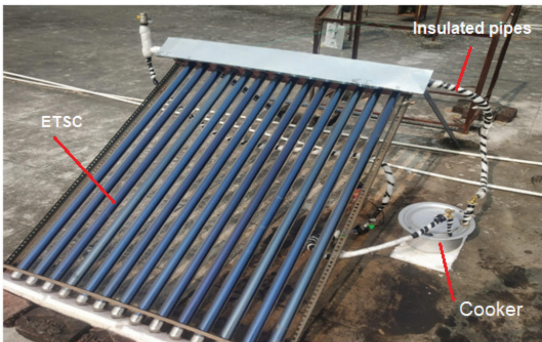
Figure 1. Evacuated tube solar cooker contains solar cooker without insulation.
