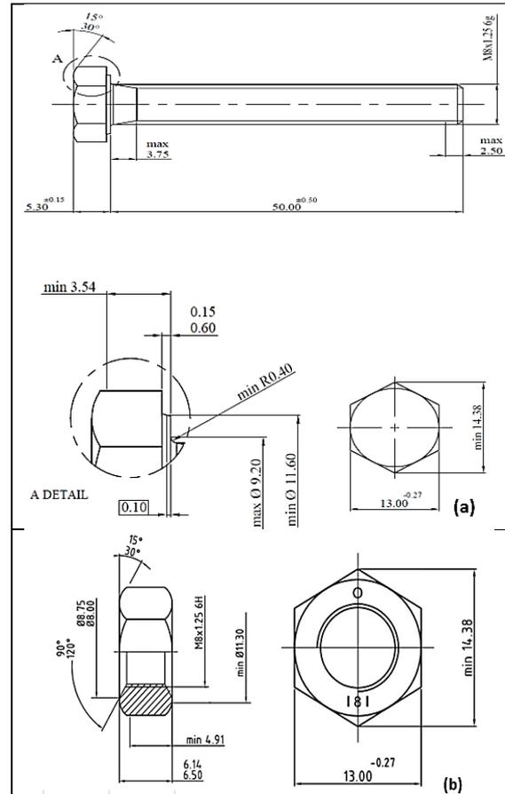
**Figure 1.** (a)Bolts Dimensions (b)Nuts Dimensions
