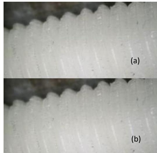
Figure 11. (a) 0/90 PET Bolt (b) -/+45 PET Bolt
