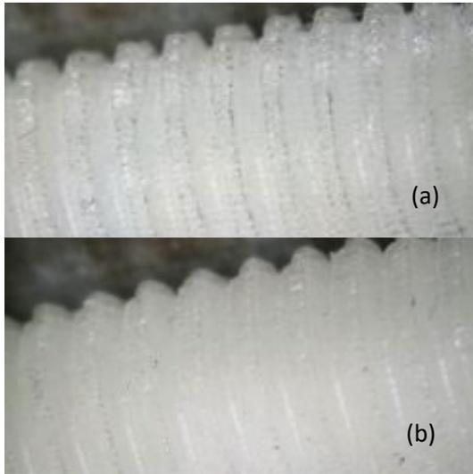
**Figure 12.** (a) 0/90 PLA Bolt (b) +/-45 PLA Bolt
