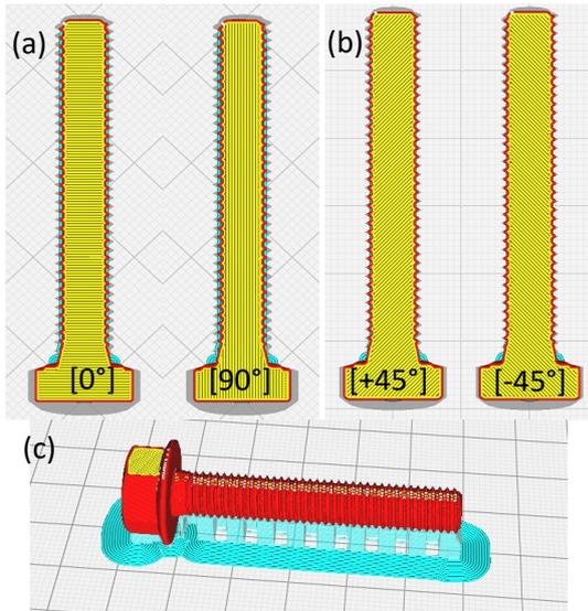
**Figure 2.** (a) Infill Patterns Angles [0/90] (b) Infill Pattern Angles [+45/-45] (c) Bed Table Position
