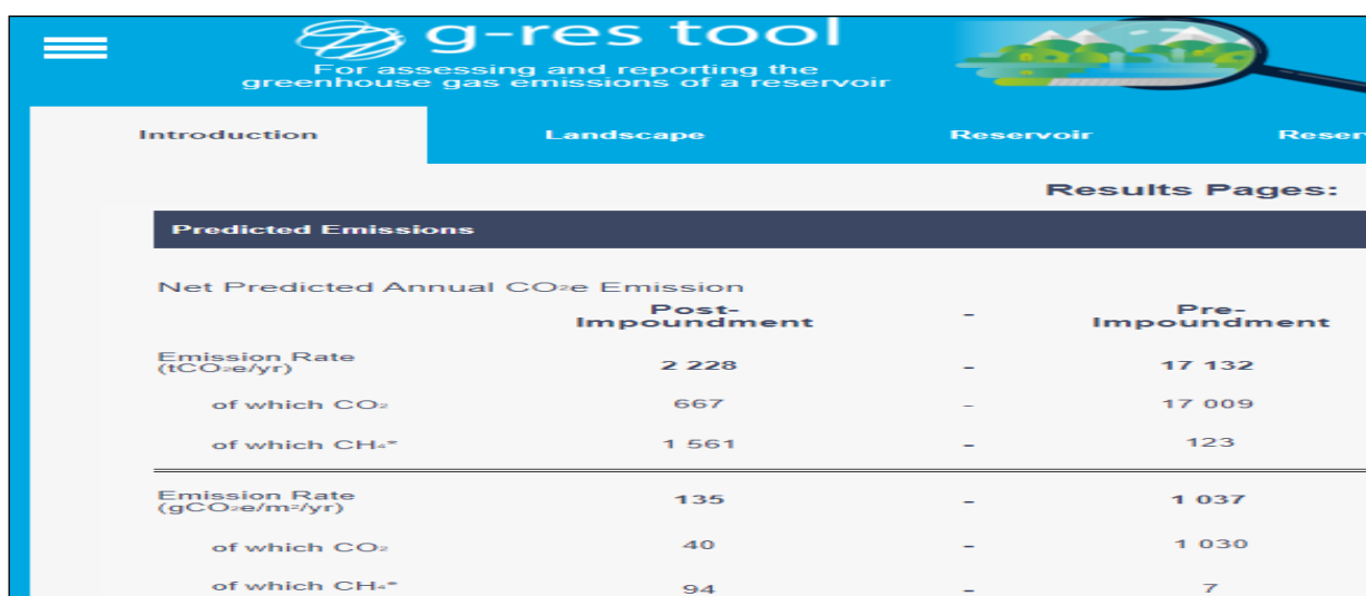
Figure 3. The GHG emission values of the Tuzluca Dam and HEPP project before and after the dam.
