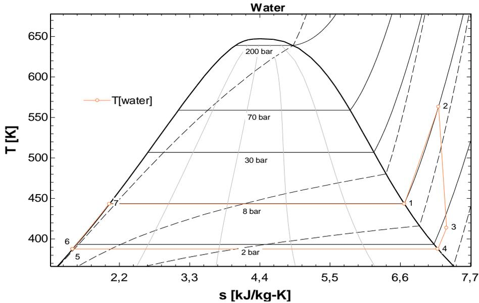
Fig. 5. Rankine Cycle temperature-entropy diagram
