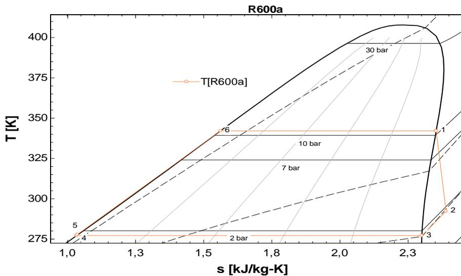
Fig. 3. Organic Rankine Cycle temperature-entropy diagram
