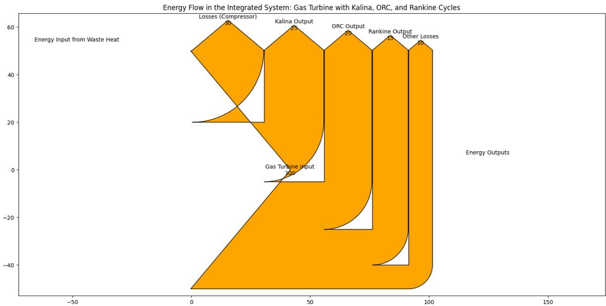
Fig. 7. Sankey diagram represents the energy flow in Kalina, ORC and Rankine cycles integrated with gas turbine
