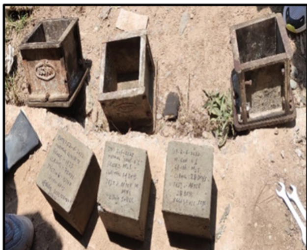
Figure 4. De-moulded concrete cubes after 24 hours
