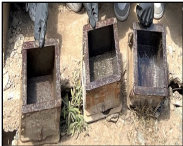
Figure 3. Moulds used for concrete cube
