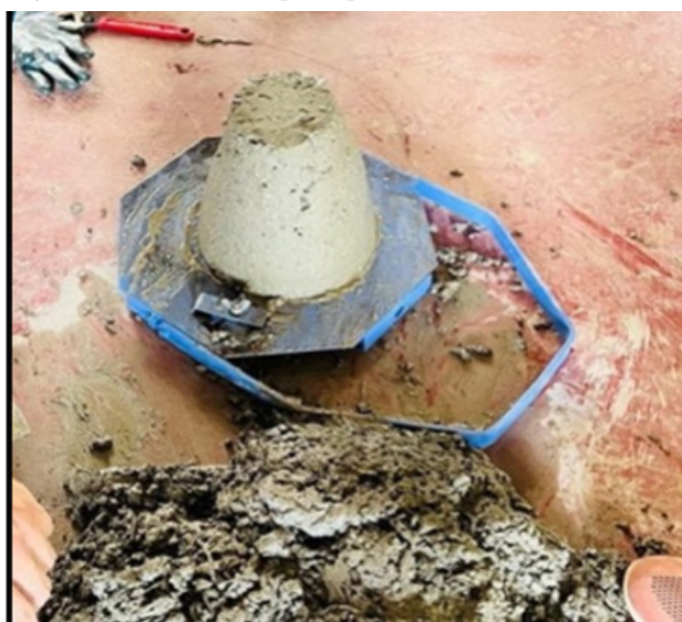
Figure 2. Measuring slump of concrete
