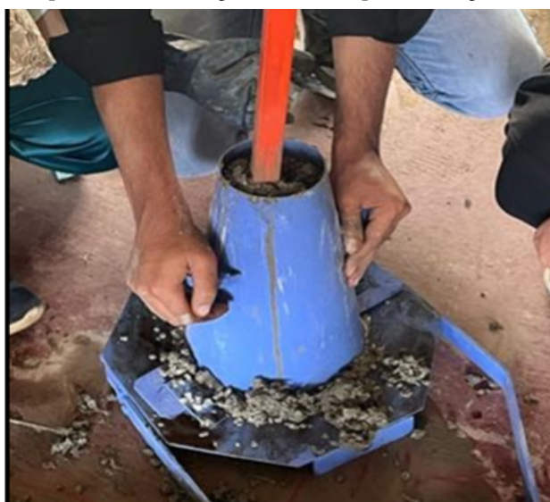
Figure 1. Concrete slump test procedure
