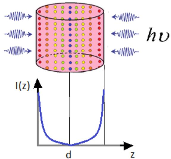
Figure 1. Schematic illustration for determining the path length of radiation in a mixture.
