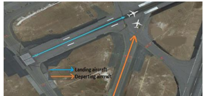
Figure 19. Runway Intersection Departure in Use
