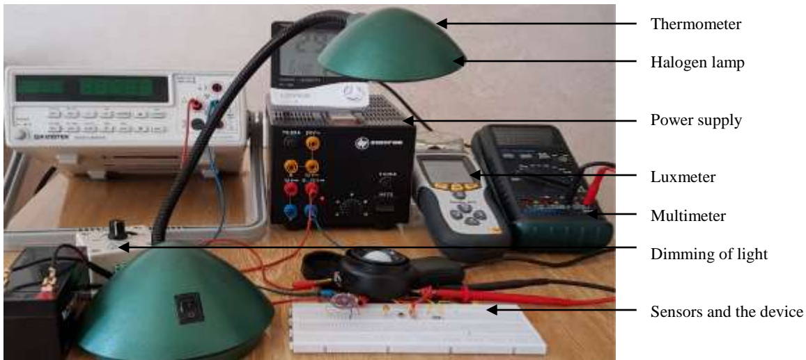
Figure 3. The System Used for Observing the Output Currents of LDR and Photodiode under Different Lighting Levels and DC Power
