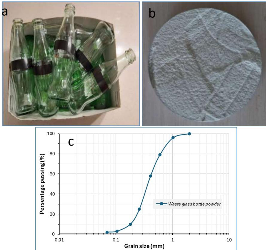
Fig. 3. Photographs, waste glass bottle (a), waste glass bottle powder (b) and granulometry curve (c)
