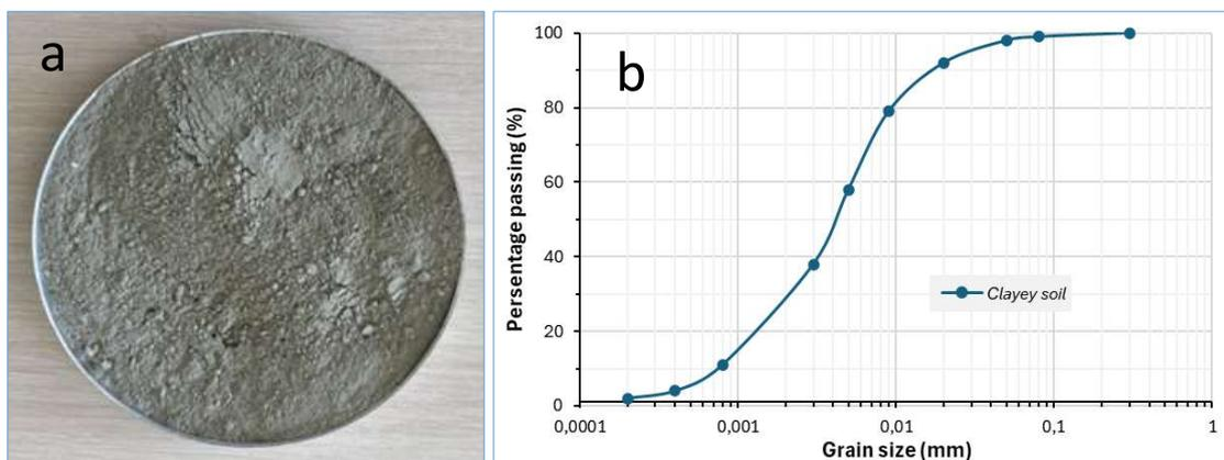
Fig. 1. Photographs, clayey soil material (a) and granulometry curve (b)
