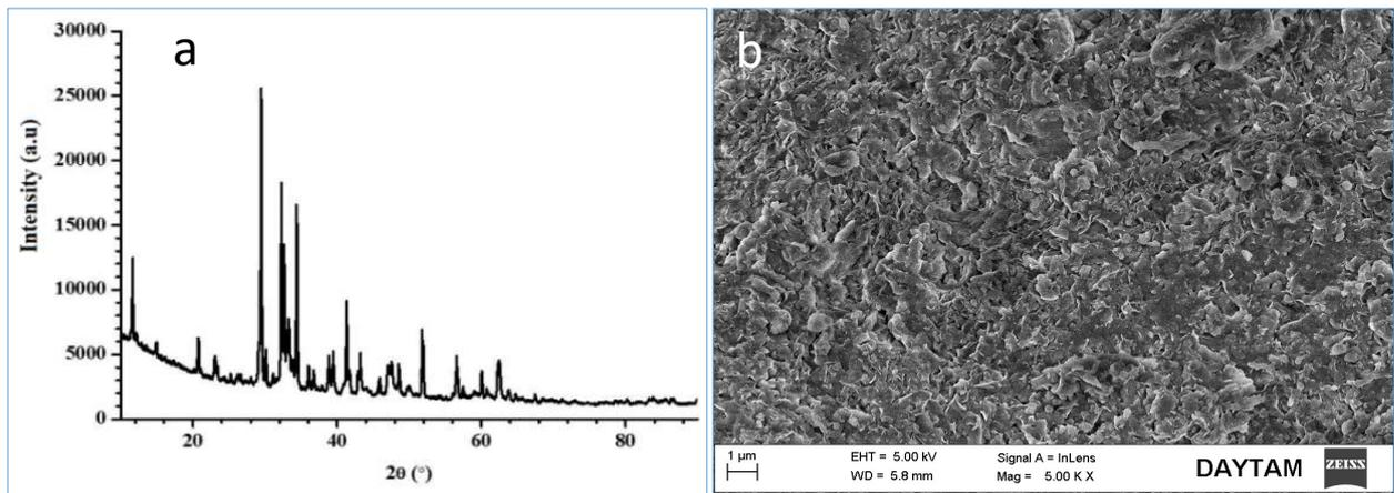
Fig. 2. XRD graph (a) and SEM pattern (b) of clayey soil
