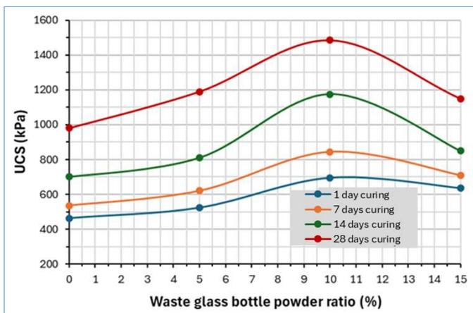
Fig. 7. Effect of curing on UCS values of stabilized with waste glass bottle powder and exposed to freeze-thaw samples
