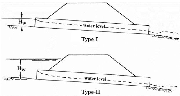
Figure 6. Operating conditions for inlet control (Type I and Type II) [4]
