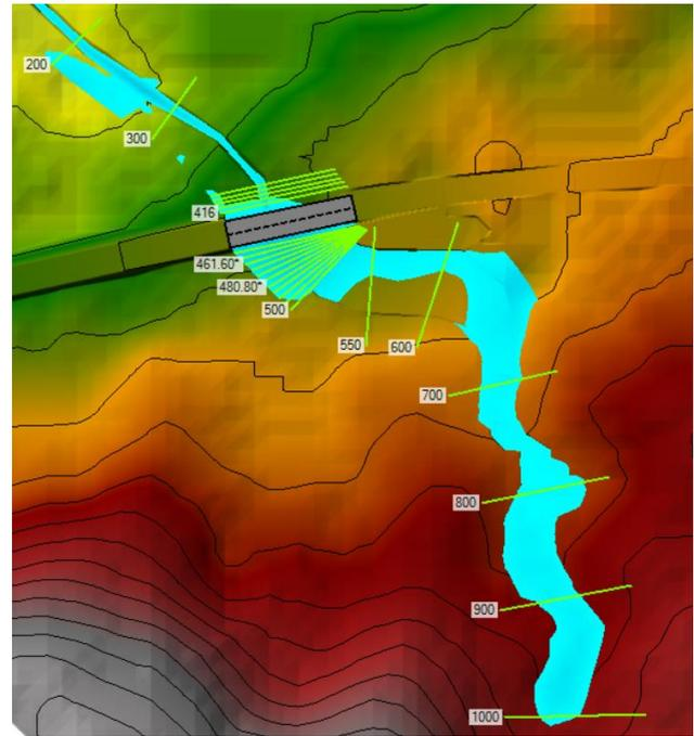
Figure 13. Ponding area for  $Q_{100}$  discharge
