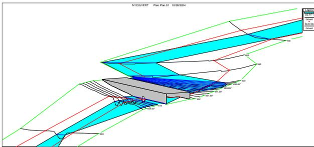
Figure 2. Perspective view of culvert for  $Q_{100}$  discharge
