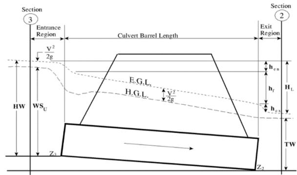
Figure 7. Typical lateral cross section of a culvert [25]
