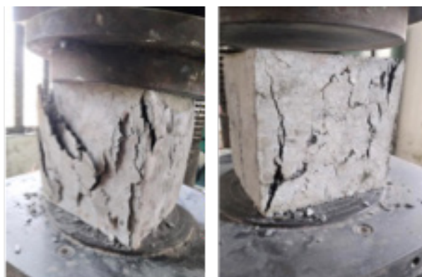
Figure 3. Mode of failure of casted cubes
