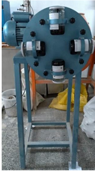
Figure 3. California stripping test device
